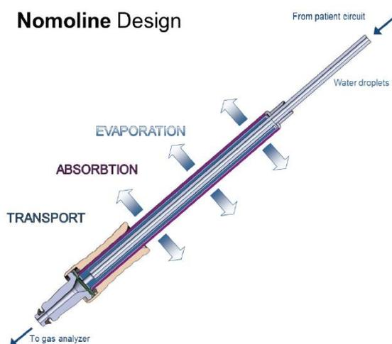
Figure 2: Nomoline Adapter
