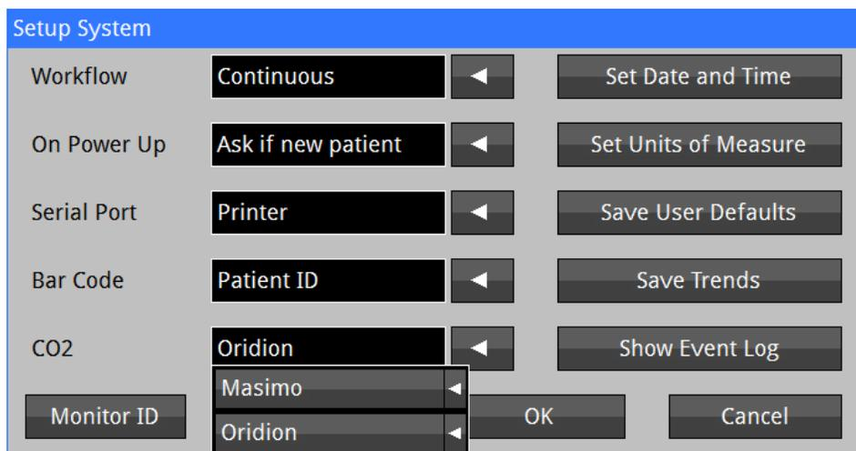
Figure 9: System Setup screen (Oridion CO<sub>2</sub> enabled)
