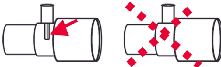
Figure 3: T-Adapter Placement
