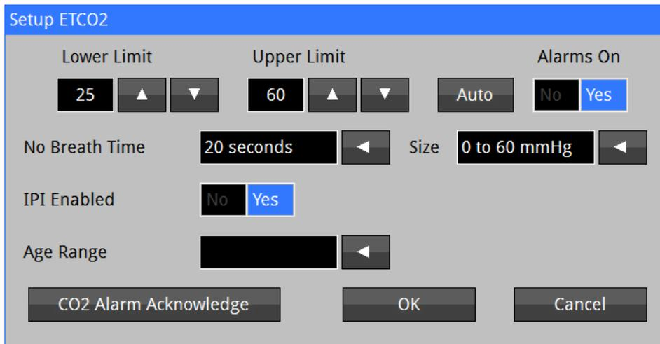
Figure 16: Oridion Setup ETCO2 Menu (w/IPI enabled) - **Pediatric Mode**
