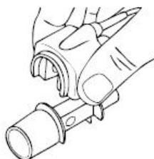
Figure 26: Snapping IRMA onto Adapter
