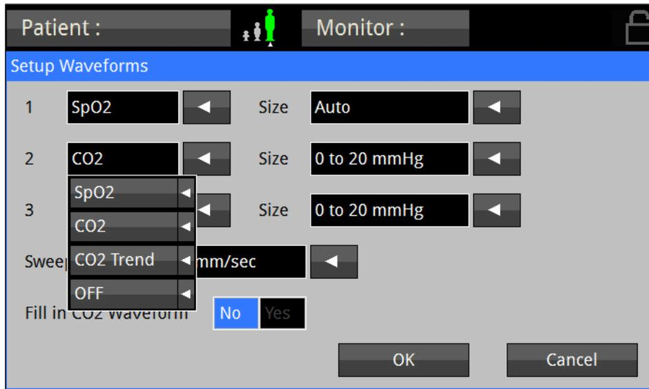
Figure 8: Waveform Setup screen (Oridion CO<sub>2</sub> enabled)
