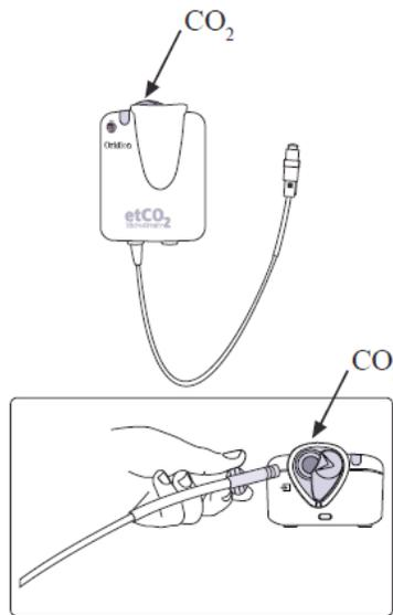
Figure 10: Inserting sample line into module
