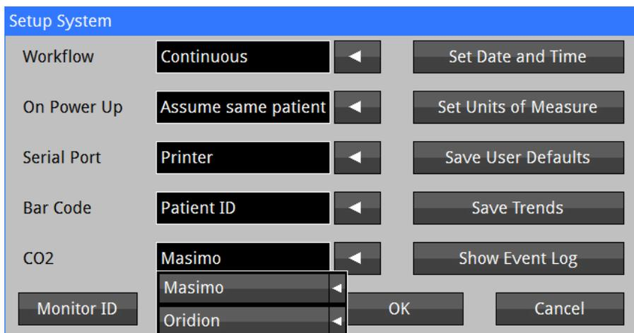
Figure 24: System Setup screen (Masimo CO<sub>2</sub> Enabled)
