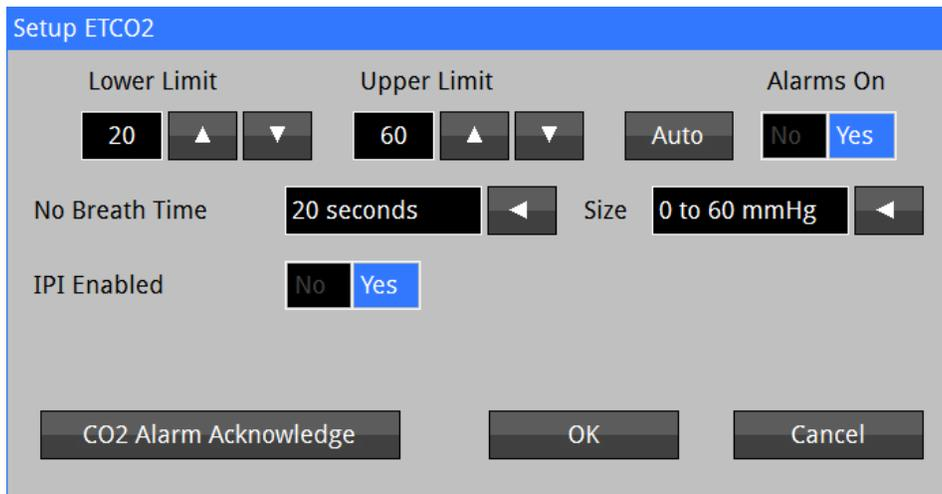
Figure 15: Oridion Setup ETCO2 Menu (w/IPI enabled) - **Adult Mode**
